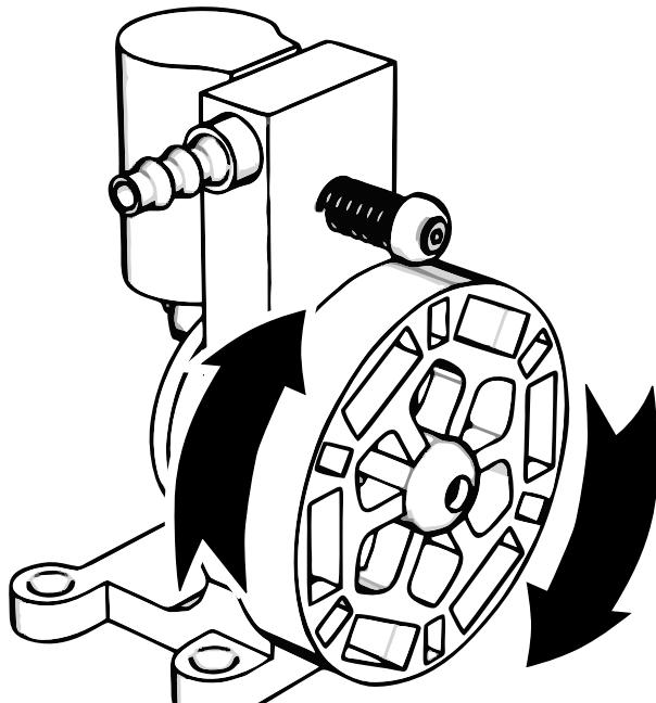
This engine is designed to run clock-wise. Attach a 1/4 inch ID hose connected to a regulated air supply to the hose barb on the engine. With the air pressure set to 10 PSI, give the flywheel a spin in a clock-wise direction. I do not recommend running at a pressure higher than 20 PSI.
